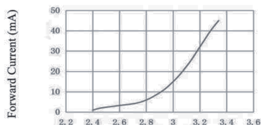
伏安特性曲线 Forward Current VS. Forward Voltag (Ta=25°C)
